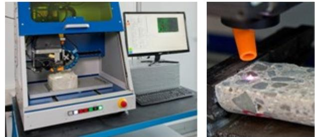
**Fig. 1.** Overall view of the LIBS laboratory system (left). Detailed view on the sample surface with plasma and nozzle of helium feeder (right).
