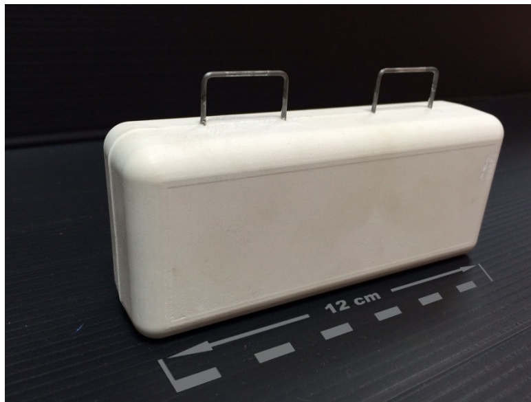
Figure 2: Sika® FerroGard® ICM discrete galvanic zinc anode (SFG-anode) for the prevention of the formation of incipient anodes induced by patch repairs
