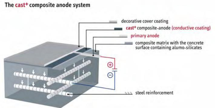
Figure 4: Schematic presentation of the CAST<sup>+</sup> composite anode system, based on the CAST<sup>+</sup> composite anode paint.
